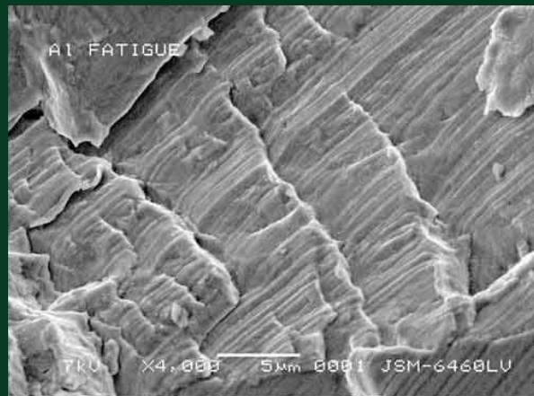
SEI, fatigue striations in fractured aluminum
