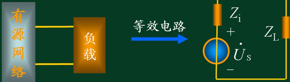
$$Z_i = R_i + jX_i, \quad Z_L = R_L + jX_L$$
