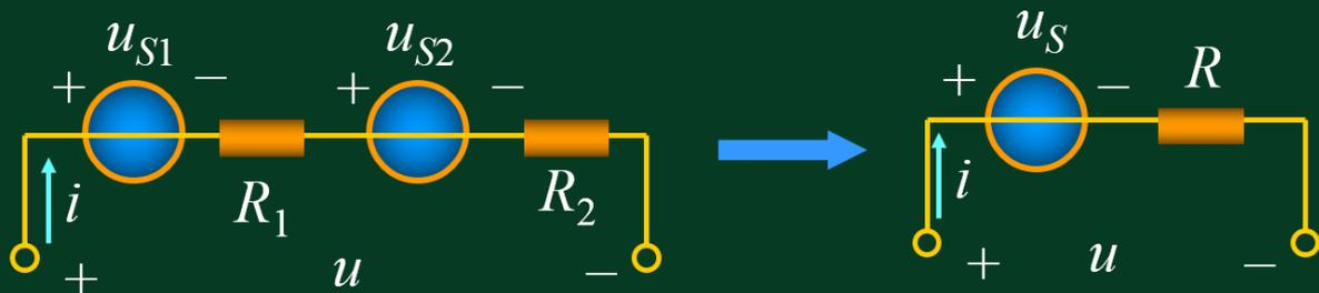
$$u = u_{s1} + R_1 i + u_{s2} + R_2 i = (u_{S1} + u_{S2}) + (R_1 + R_2) i = u_S + Ri$$
