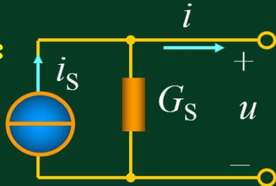
$$i_s = u_s / R_s, \quad G_s = 1 / R_s$$
