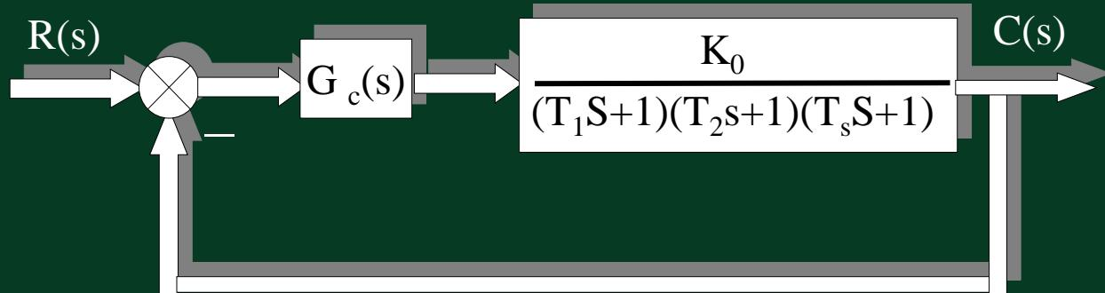
$$T_1 = 0.049 \quad T_2 = 0.026 \quad T_s = 0.00167 \quad K_0 = 55.58$$
