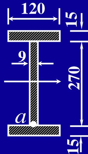
$$\sigma = \frac{M_{\max} \cdot y_a}{I_z} = \frac{(80 \times 10^3 \text{ N} \cdot \text{m})(135 \times 10^{-3} \text{ m})}{88 \times 10^{-6} \text{ m}^4} = 122.7 \text{ MPa}$$
