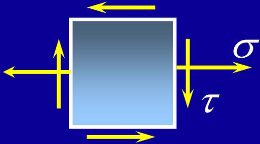
$$\begin{aligned}\sigma_{r3} &= \sigma_1 - \sigma_3 = \sqrt{\sigma^2 + 4\tau^2} \\ &= \sqrt{122.7^2 + 4 \times 64.6^2} \\ &= 178.1 \text{MPa}\end{aligned}$$
